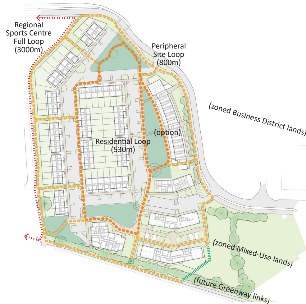
Diagram illustrating the intention for designed loop walks (and their associated distances). The aim is to provide routes that are easy to navigate and allow for integration with future development lands and Greenway links.
